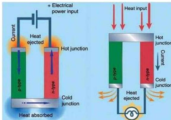
A third alternative uses thermo-electric effect to generate a small but usable amount of electricity using the thermal gradient of the pavement infrastructure which can satisfy the lighting needs on the road.
