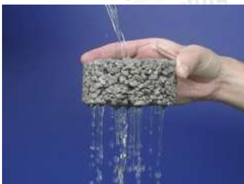
Fig.No.3 Free Draining of porous concrete.
