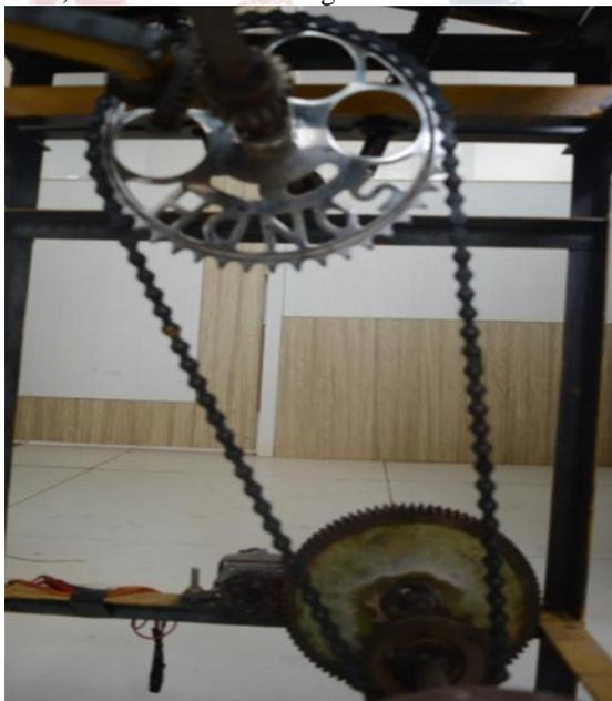
Fig. 1 Chain Sprocket Arrangement
