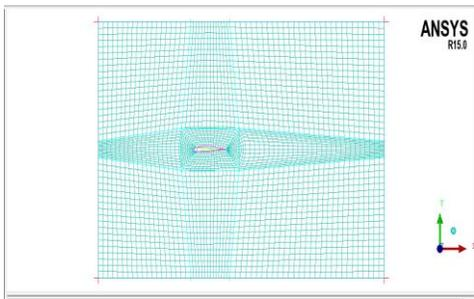
Fig 13: meshing of Modified NACA2412 Aerofoil
