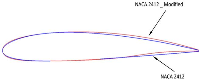
**Fig7: Base NACA 2412 aerofoil and modified NACA 2412 aerofoil**
