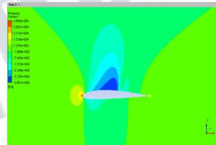
Fig 15: result for pressure Aerofoil NACA2412
