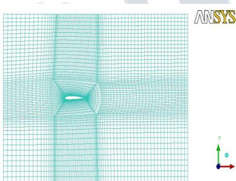
Fig 10: meshing of NCA2412 Aerofoil
