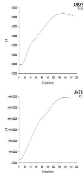
Fig21: lift coefficient for NACA2412 aerofoil and modified NACA2412 aerofoil.
