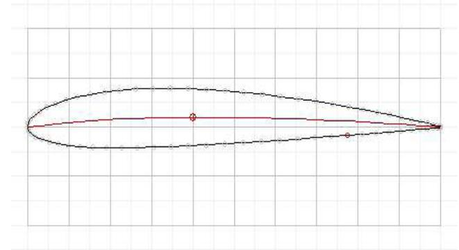
Fig 6: NACA 2412 Aerofoil Station
