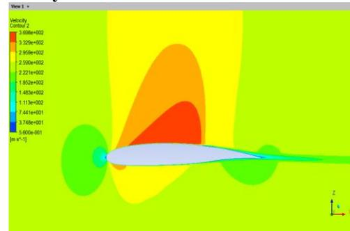
Fig 19: result for velocity Aerofoil modified NACA2412
