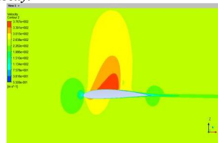
Fig 16: result for velocity Aerofoil NACA2412
