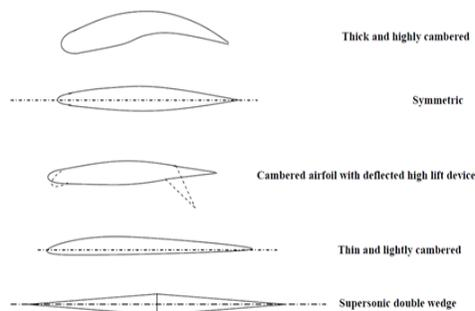
Fig 5: Five sample Aerofoil section
