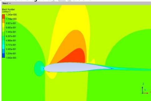
Fig 17: Result for mach Aerofoil modified NACA2412
