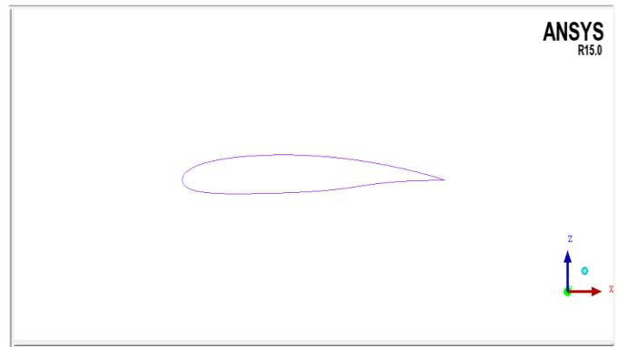
Fig 11: Model modified NACA 2412 Aerofoil
