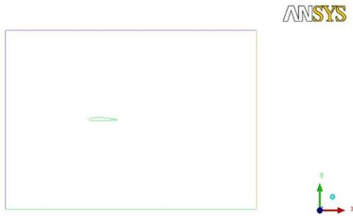
Fig 9: domain over Model NACA 2412 Aerofoil
