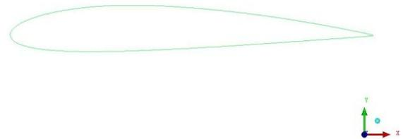
Fig 8: Model NACA 2412 Aerofoil
