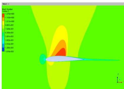
Fig 14: Result for mach Aerofoil NACA2412
