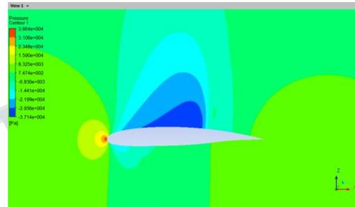
Fig 18: Result for pressure Aerofoil modified NACA2412
