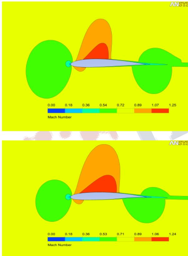
Fig 20: Mach contour on NACA2412 and NACA2412\_modified (M = 0.75) and the pressure distribution
