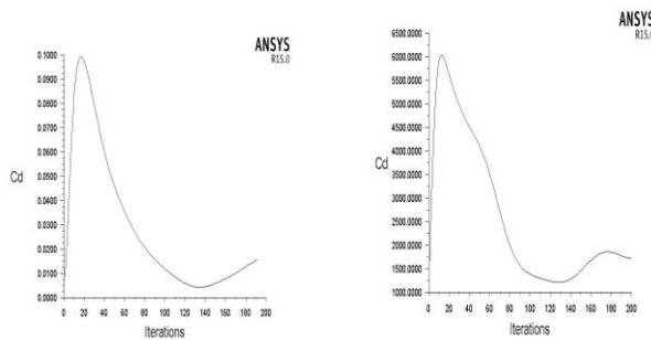
**Fig22: drag coefficient for NACA2412 aerofoil and modified NACA2412 aerofoil.**
