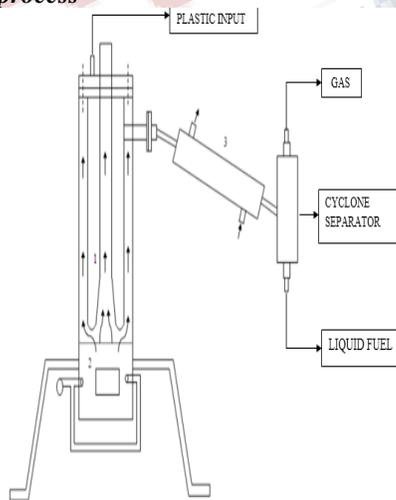
1. Reactor, 2. Combustion chamber, 3. Condenser
