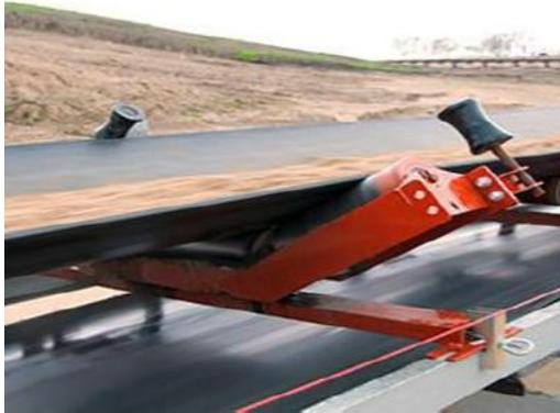
**Fig 2.1 Self alignment pulleys**
