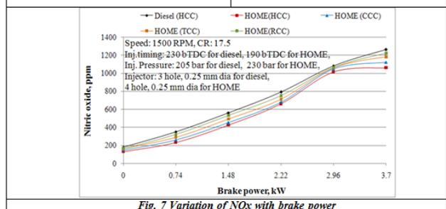
Fig. 7 Variation of NO<sub>x</sub> with brake power
