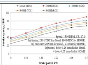
Fig. 4 Variation of smoke with brake power
