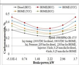
Fig. 6 Variation of CO with brake power
