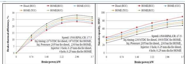
Fig. 3 Variation of BTE with brake power
