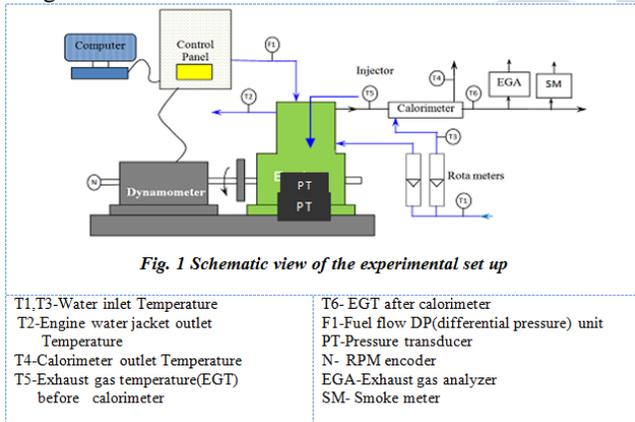
Fig. 1 Schematic view of the experimental set up
