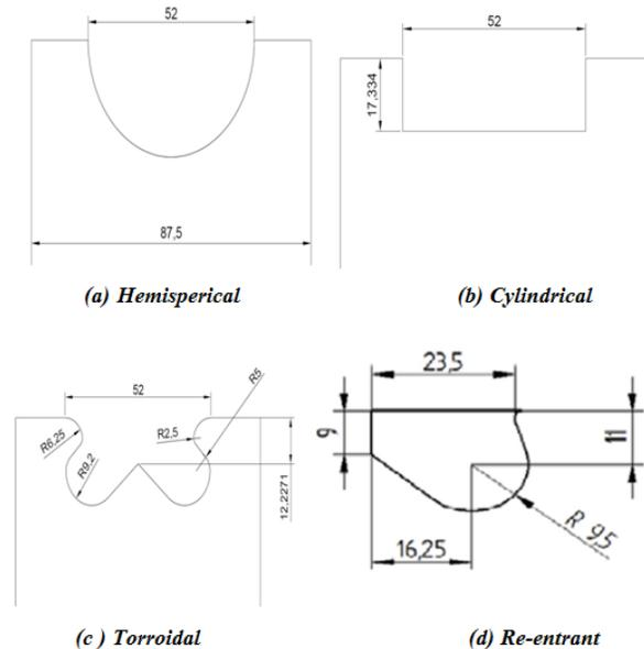
Fig. 2 Combustion chambers used in the present work
