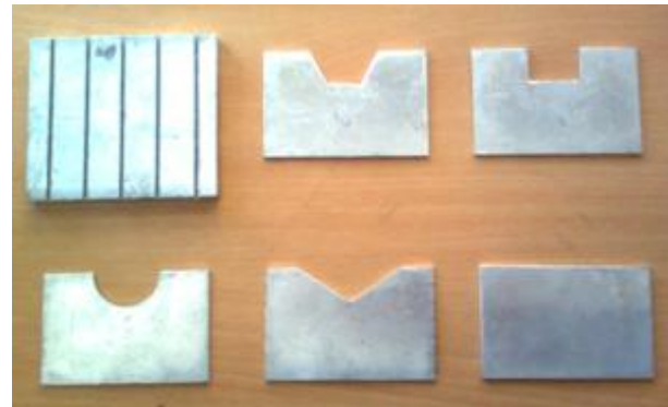
Fig 2: Base Plate With Different Types Of Fins
