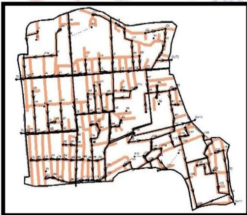
Fig 4. Map with all conduits of drainage system
