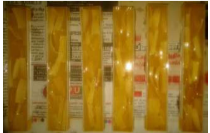
Figure :3 Prepared composite through hand layup process
