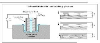
Fig. 1: Principle of Electrochemical Machining
