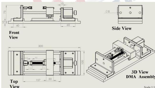
**Figure.1 Computer Aided Drafted view of DMA system.**
