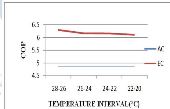
The above figure 3 deals with the comparison of COP between air cooled(AC) condenser and evaporatively cooled condenser(EC) for flow rate 8.5 L/min and temp 35 °C . It can be seen that EC has higher COP than AC. for EC and AC decrease in temperature range decreases the COP.
