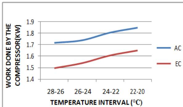
**Fig 1 Temperature Interval vs. Work done by compressor**
