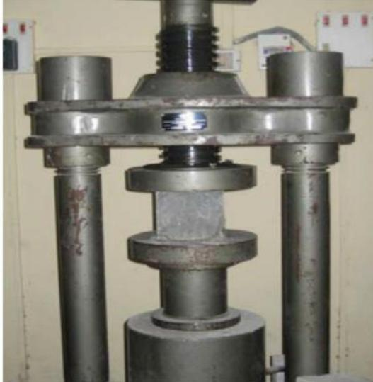
**Figure 2 :- Test for Compressive strength.**
