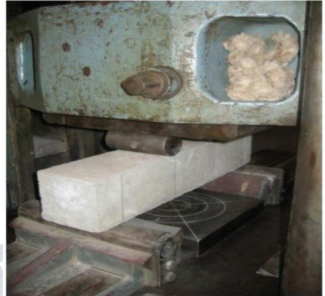
**Figure 3 :- Test for Flexural Strength.**
