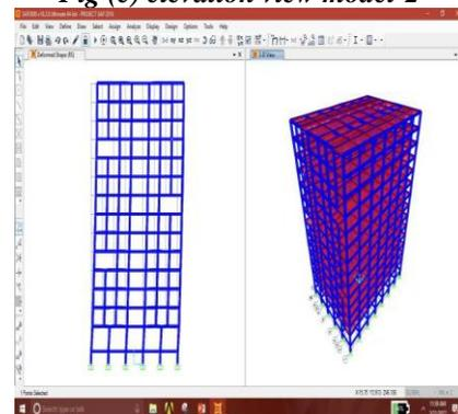
*Fig (f) deformed shape of the structure model-2*
