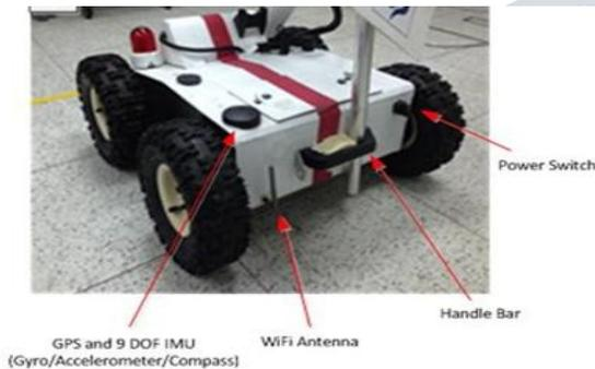
**Fig. 4. System structure of Ambulance Robot**
