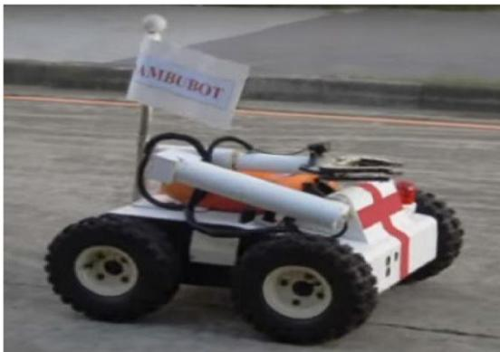
**Fig. 2. The developed Ambulance Robot.**
