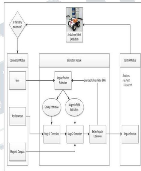
**Fig. 10. Sensor fusion architecture of ambulance robot.**
