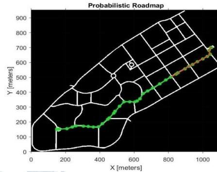
**Fig. 14. The Probabilistic Roadmap calculated by Ambubot**
