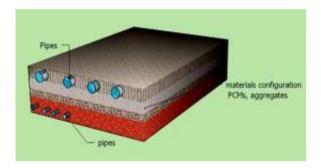
Another practical approach to harvest solar energy from pavements is to embed water-filled pipes beneath the asphaltic segment of the road and allow the sun to warm the water.
