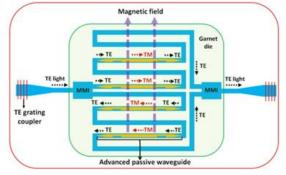
Fig.1: Design of Optical Isolator
