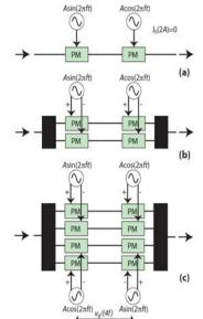
Fig.2: Tandom Phase Modulator. (a) single arm (b) two arm (c) four arm
