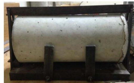
Figure 4: Cylinder Placed in the Steel Strips
