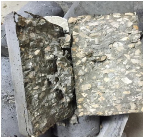
Figure 14: Non Rubberized Concrete Cylinders Splitting into Two Halves.
