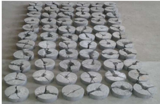
Figure 9: Portion of the Specimens Subsequently to Impact Load Failure
