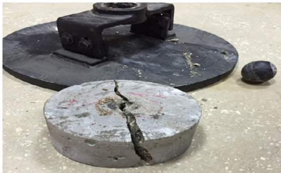
Figure 7: Rubberized Concrete Impact Failure
