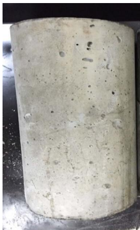
Figure 15: Rubberized Concrete Cylinders without Splitting After Failure
