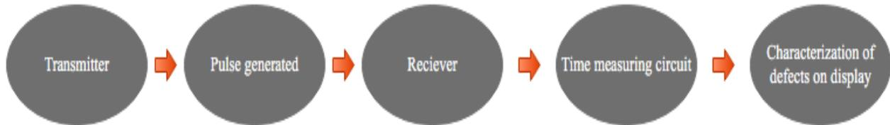
**Systematic Process of Ultrasonic process**
