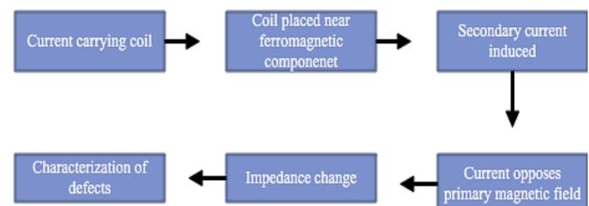
**Eddy Current Testing-** Eddy current is a nondestructive testing technique which works on the principle of electromagnetic induction [6]. This technique is mainly used to detect flaws, depth of defect in the conducting materials
