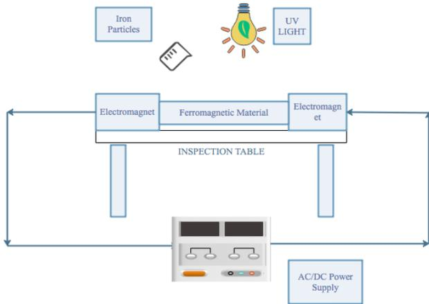
**Figure 3: Magnetic Particle Testing [16]**
