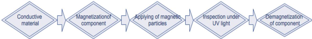
**Systematic process of Magnetic particle testing**
