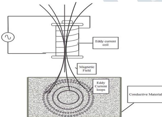
**Figure 1: Eddy current testing [17]**
