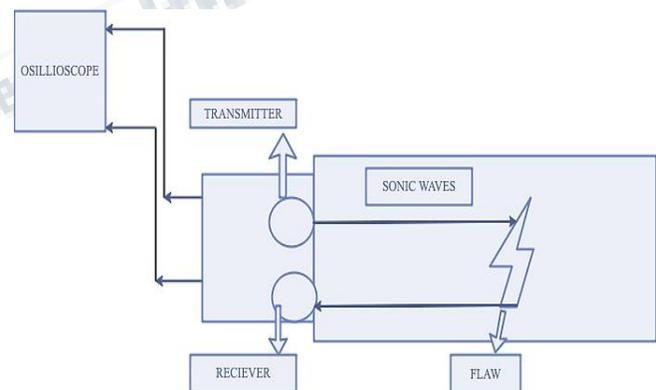
**Figure 2: Ultrasonic Testing [14]**
