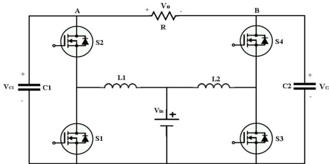
**Fig.1. DC-DC-AC converter**
