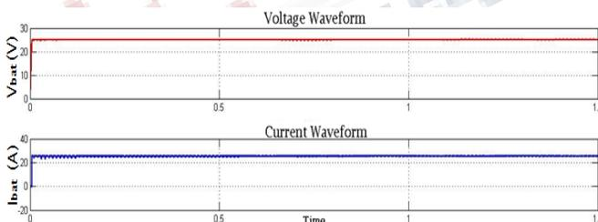
**Fig.7. Battery Charging Voltage and Current Waveforms At 1000W/m<sup>2</sup> Irradiance During IBC mode**
