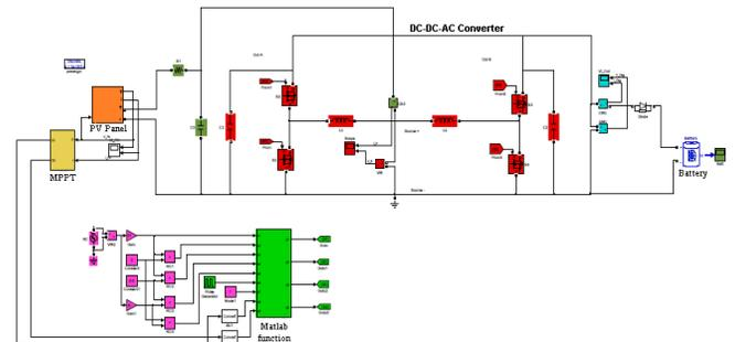
**Fig.3. MATLAB/Simulink Model of Photovoltaic Fed Battery Charging System Using DC-DC-AC Converter**
