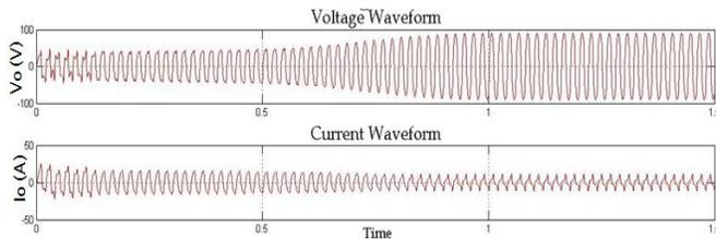
**Fig.5. DC-DC-AC converter Output Voltage and Current Waveforms During DBI Mode**
