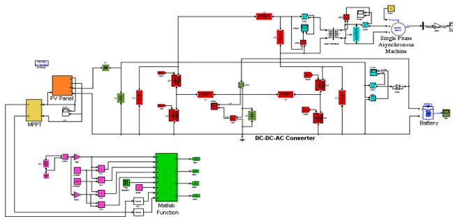
**Fig.4. MATLAB/Simulink Model of Combined Photovoltaic and Battery Fed Induction Motor Drive Using DC-DC-AC Converter**
