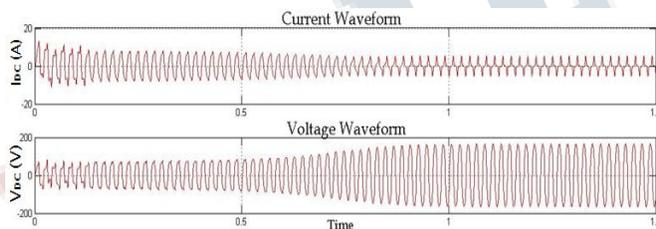
**Fig.6. Single Phase Induction Motor Output Voltage and Current Waveforms**
