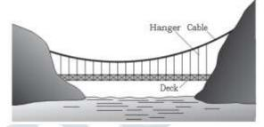
Consider the suspension bridge as shown, which consists of the main cable, the hangers, and the deck. The self-weight of the deck and the loads
