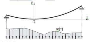
applied on the deck are transferred to the cable through the hangers.
