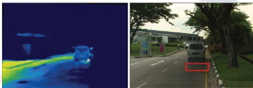
Fig. 2. An example of smoke detection on a small road section with HSU > 90
