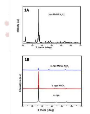
Fig.1(A) X-ray diffraction patterns of RGO/MoO<sub>3</sub> and in Fig 1 (B) pattern (a) for RGO, (b) for pure MoO<sub>3</sub> and (c) for RGO/MoO<sub>3</sub>.
