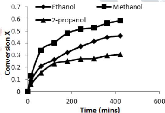
**Fig.3 Effect of varying the type of alcohols used. Reaction condition: RE/A = 1; HCl as catalyst; temperature = 333.15 K.**
