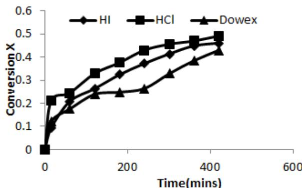
**Fig.1 Effect of the different types of catalyst used for the esterification reaction. Reaction condition: RE/A = 1; temperature = 333.15K.**
