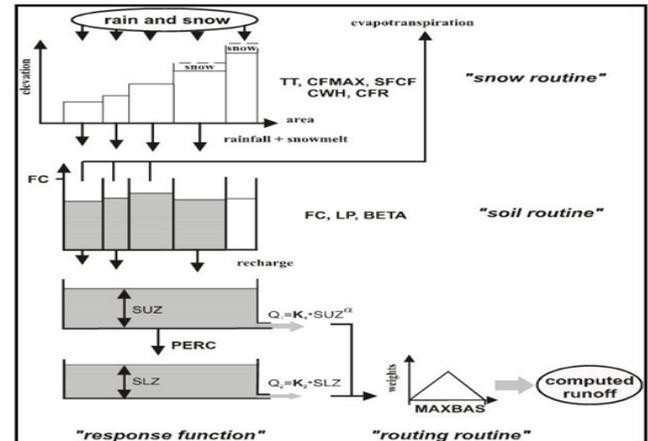
**Fig. 4 Structure of HBV model (taken from help menu of HBV – Light v4.0.0.10). Notations have been described in the text.**
