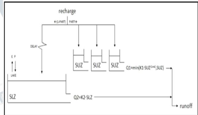
**Fig. 5 Response function module of HBV model (taken from help menu of HBV – Light v4.0.0.10). Note that this sub-model has distributed structure. Notations have been described in the text.**
