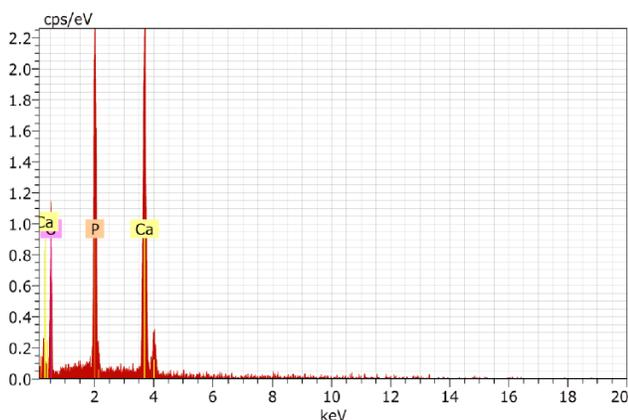
**Fig 7: EDS Spectrum of Hap**
