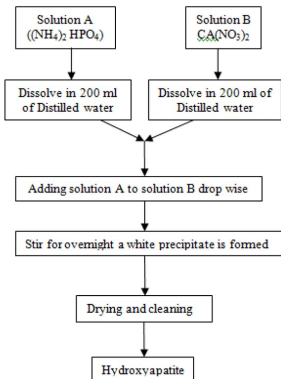
*Fig 1: Flowchart for Synthesis of HAp*
