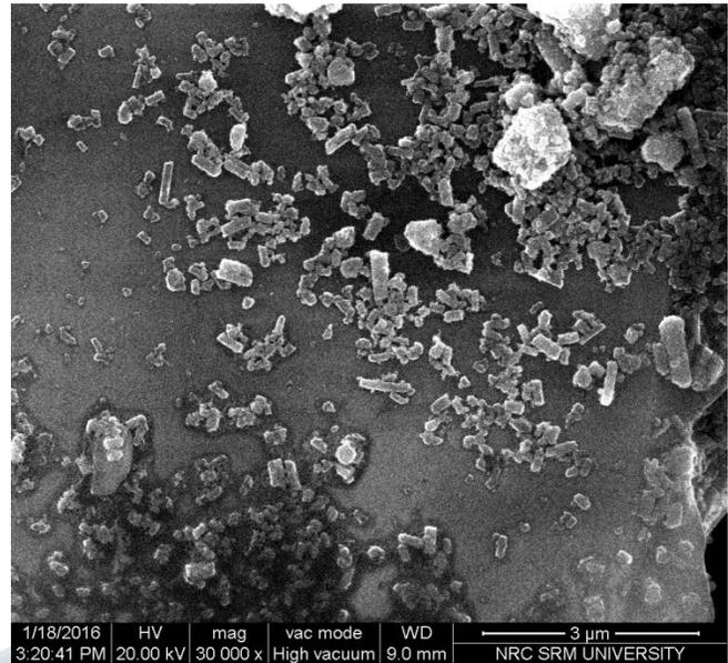
**Fig 5: SEM Micrograph of HAp of 30,000 x**
