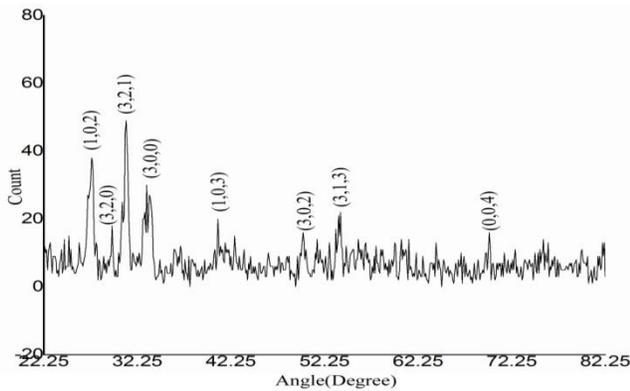
**Fig 3: XRD Spectrum of HAp**
