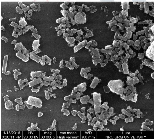
**Fig 4: SEM micrograph of HAp of 60,000x**
