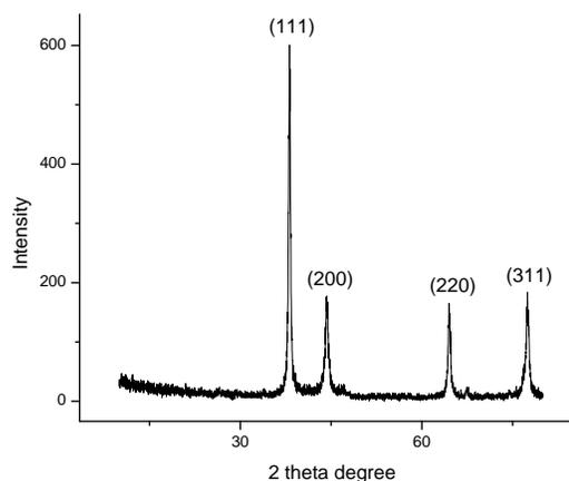
(Figure 3) XRD pattern of synthesized silver nanoparticles
