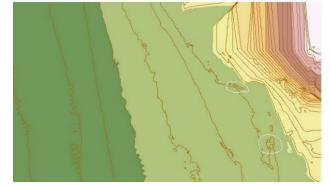
The ArcGIS 3D analyst module was used to flash a light source over the DEM at two distinct heights and azimuths in order to prepare the shaded relief images using MBES-DEM data. Depending on the elevation of the seabed topography, shadows were produced in the DEM, exaggerating the relief
