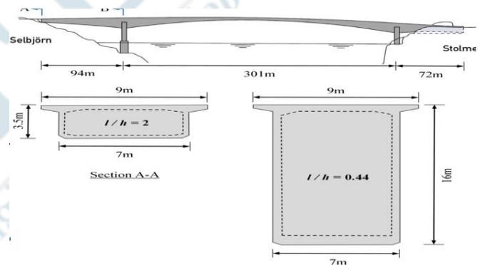
**Figure 1:** Box Girder Diaphragm Segment
