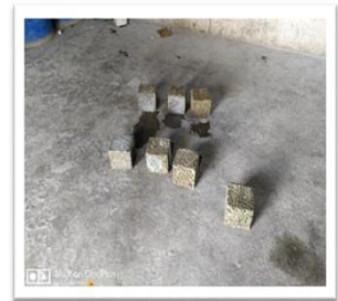
Moulded Cubes kept for 24 hours Demoulding of cubes
