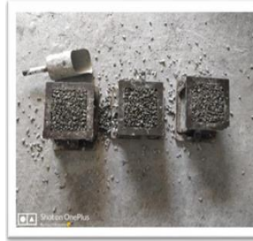
Moulded Cubes kept for 24 hours Demoulding of cubes
