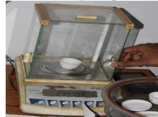
Fig.2. Digital weighing machine and crucible
