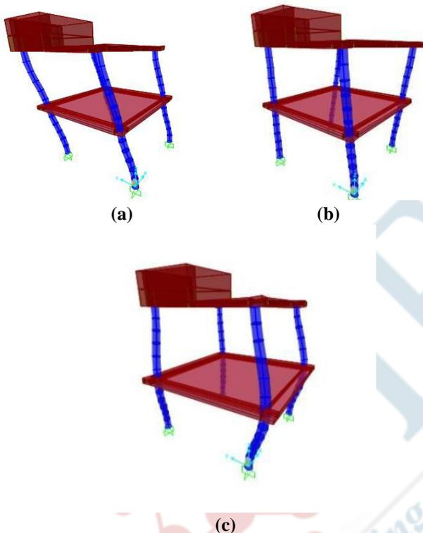
**Figure 2.** (a) 2nd, (b) 3<sup>rd</sup>, and (c) 5th modes of the numerical model
