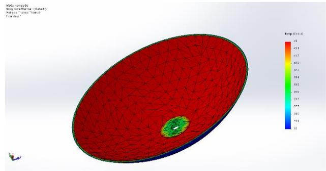
**Figure 3(a): Thermal analysis of parabolic dish**
