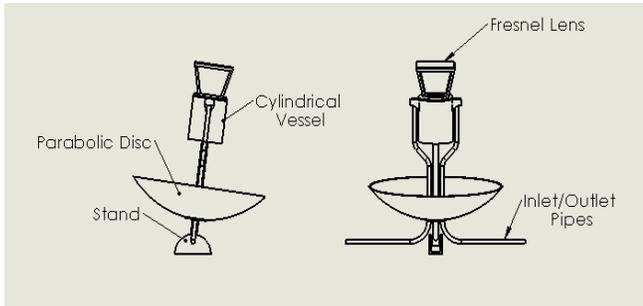
**Figure 1: Setup with labelled components**
