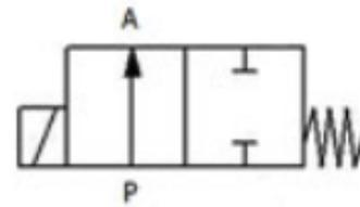
**Fig.5: Circuit Diagram of 2/2 Valves.**
