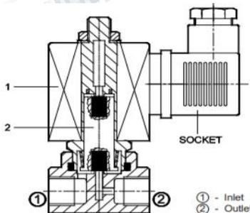
**Fig.4: Cross-Sectional View of Janatics 2/2 Valve**
