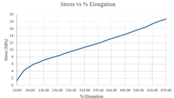
**Fig-2. Stress vs Elongation graph for seal**
