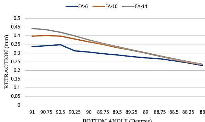
**Fig-6. Retraction vs Bottom Angle for  $45^\circ$  Corner Break Angle**
