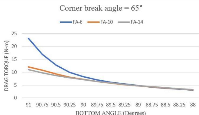
**Fig-15. Drag torque vs Bottom Angle for 65° Corner Break Angle**
