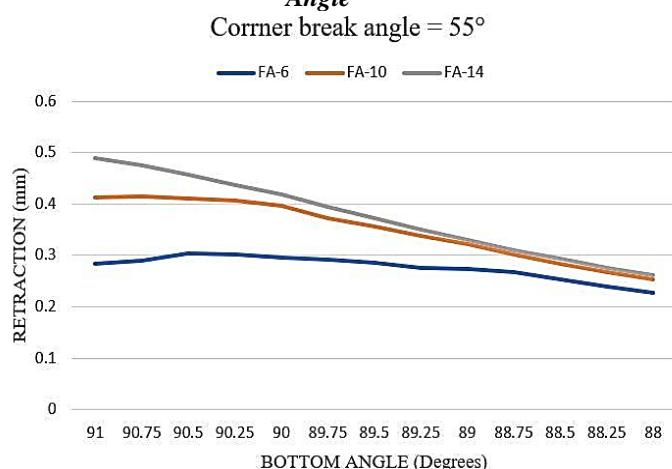
**Fig-8. Retraction vs Bottom Angle for  $55^\circ$  Corner Break Angle**
