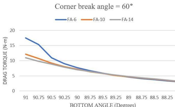
**Fig-14. Drag torque vs Bottom Angle for 60° Corner Break Angle**
