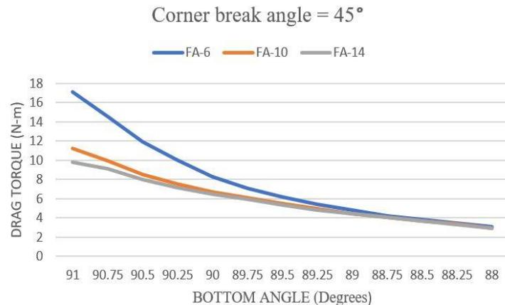
**Fig-11. Drag torque vs Bottom Angle for  $45^\circ$  Corner Break Angle**
