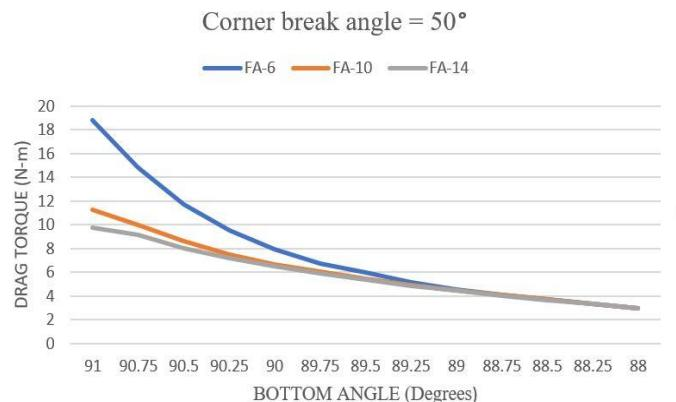
**Fig-12. Drag torque vs Bottom Angle for  $50^\circ$  Corner Break Angle**
