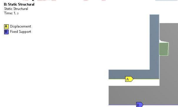
**Fig-4. Boundary Conditions for seal groove**
