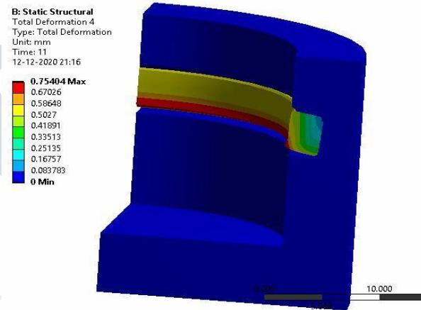
**Fig-5. Deformation of seal**
