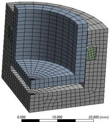
**Fig-3. Mesh for seal groove**
