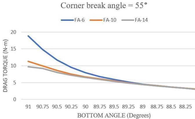
**Fig-13. Drag torque vs Bottom Angle for 55° Corner Break Angle**
