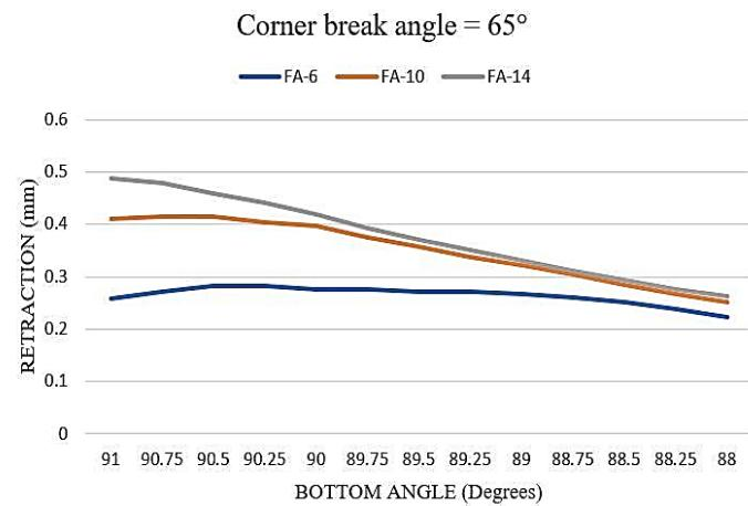
**Fig-10. Retraction vs Bottom Angle for  $65^\circ$  Corner Break Angle**
