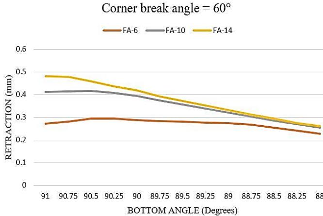
**Fig-9. Retraction vs Bottom Angle for  $60^\circ$  Corner Break Angle**
