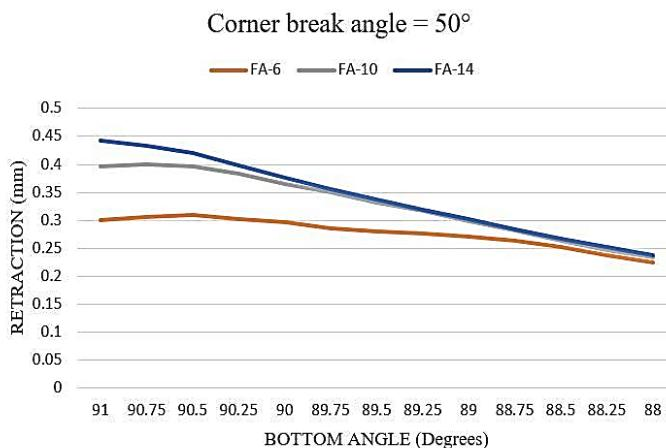
**Fig-7. Retraction vs Bottom Angle for  $50^\circ$  Corner Break Angle**
