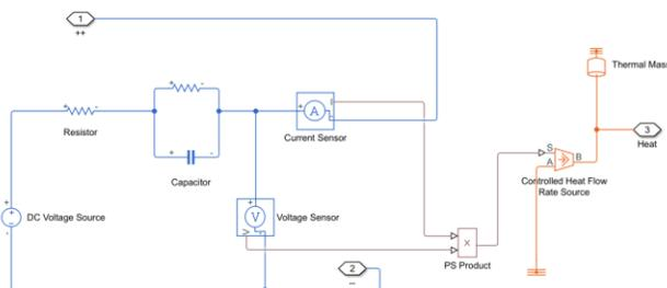
**Figure 5: Battery model**
