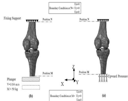
Figure 14 .Boundary conditions for free fall
