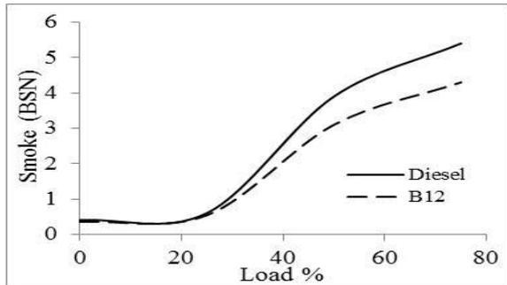
**Fig. 7 Variation of Smoke intensity with Load**
