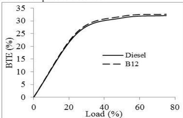
**Fig. 3 Variation of BTE with respect to Load**
