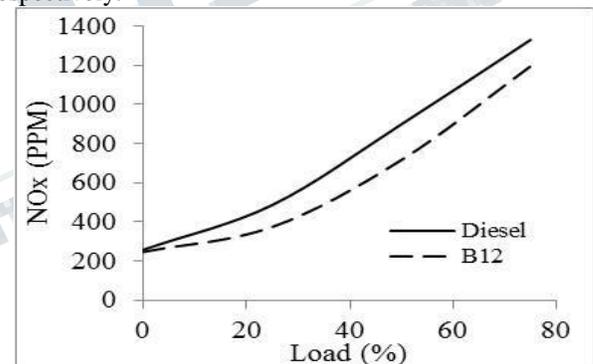
**Fig. 6 Variation of NOx emissions with respect to Load**
