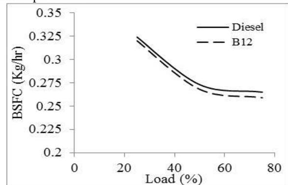
**Fig. 2 Variation of BSFC with respect to Load**
