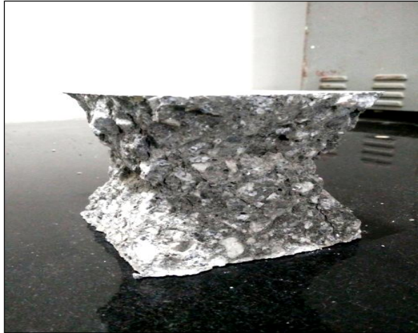
Fig 2: Failure pattern of cubes tested for compressive strength
