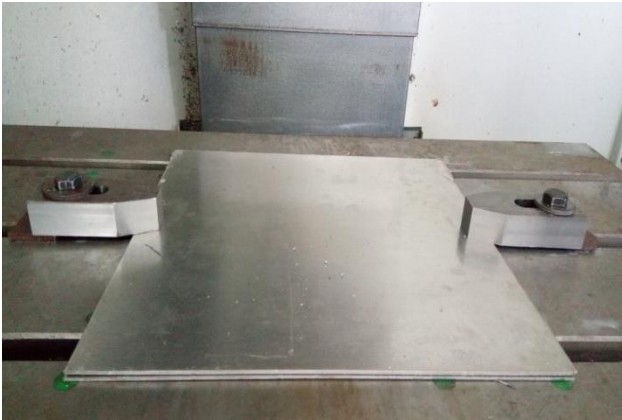
Figure-4: Use of Fixture for sheet metal application
