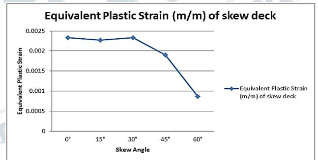
**Fig 4: Variation of Equivalent Plastic Strain vs Skew angle.**
