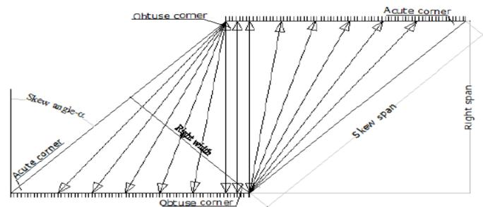
**Fig 1: Basic structure of a skew slab**
