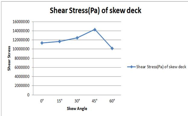
**Fig 6: Variation of Shear Stress vs Skew angle.**
