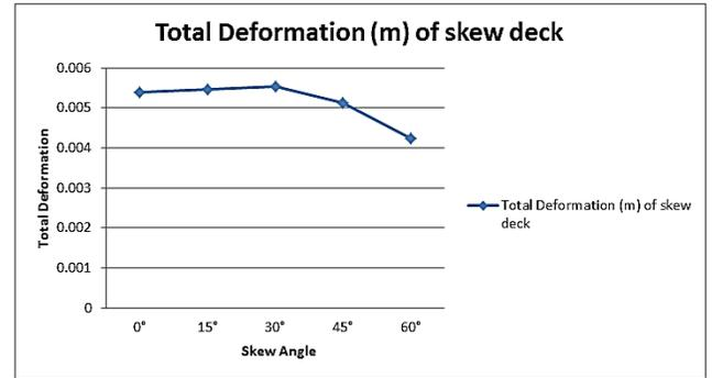
**Fig 3: Variation of Total Deformation vs Skew angle.**
