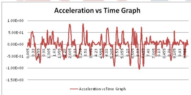
**Fig 2: Graph showing the acceleration vs time variation for the Bhuj earthquake.**
