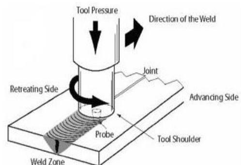
**2.1 Mechanism of Joining in FSW**
