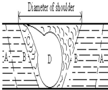
**Figure 2: Schematic cross-section of a typical FSW weld showing four distinct zones.**
