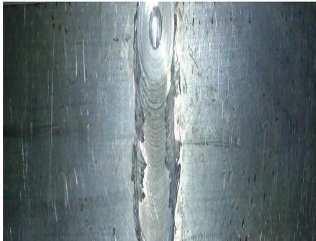
**Figure.8 Welded Specimen at 1200 rpm**
