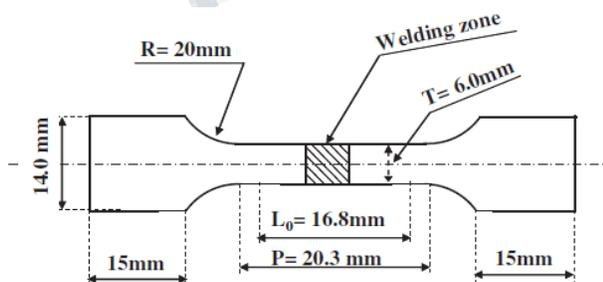
**Figure.9 Tensile Test Specimen Dimensions**
