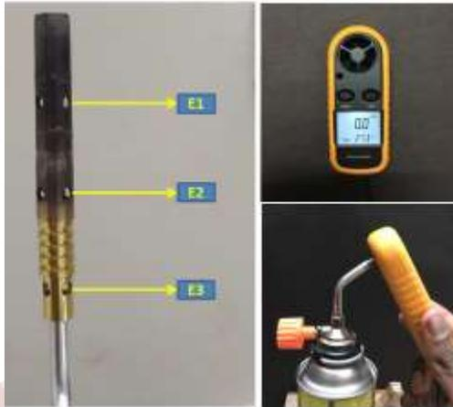
Fig. 3 (a): Air-entraining holes Fig. 3(b): Anemometer
