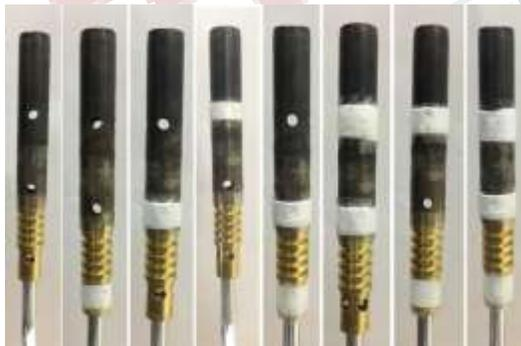
Fig. 4: Cases of various combination of location of air-entrainment enclosure area by enclosing holes: (a) All holes open, (b) only E3 closed, (c) only E2 closed, (d) only E1 closed, (e) only E1 open, (f) only E3 open, (g) only E2 open and (h) All closed.
