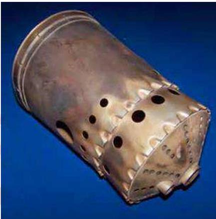
*Fig. 31 (a): Combustion Chamber*
