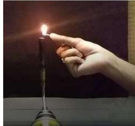
Fig. 5: Enlighting the burner from the top opening of the burner by a matchstick
