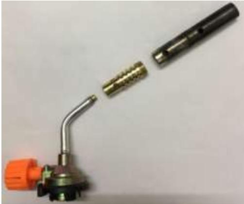
Fig. 2: Removable sub-parts of nozzle
