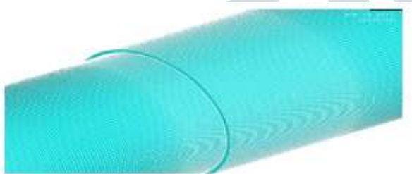
Figure 1. Zoomed View of FE Model of Tubular Lap Joint
