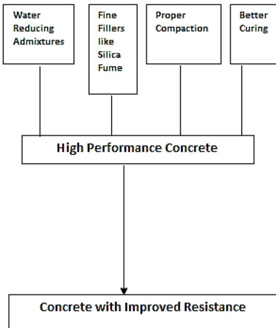
Figure 1: Reduction of Capillary Pore Size for Production of HPC.
