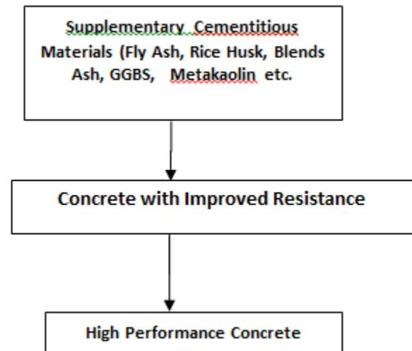
Figure 2: Role of Chemically Active Binding Agents to Improve Resistance of concrete.
