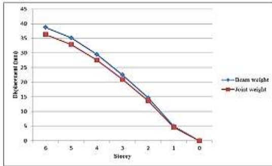
Fig. 4. Storey displacement in Z in mm
