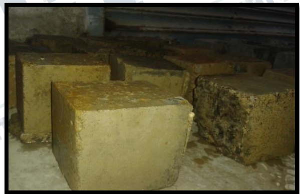
Fig-2-Specimens after HCL Attack
