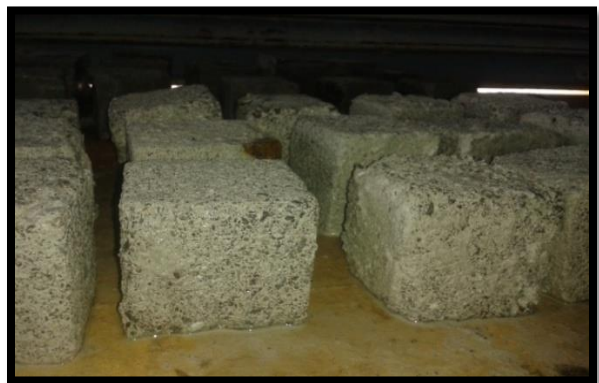
Fig-3- Specimens after H2So4 Attack
