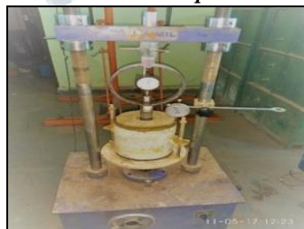
Fig. 4.1.3: Set up for Swelling Pressure Test
