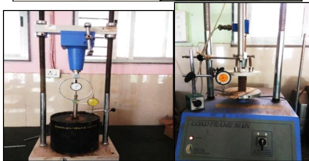
(a) Sample Wrapped in Polythene Bag (b) Desiccator (c) UCS Test Set up
