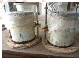
Fig. 4.1.2: CBR Samples Kept for Curing and CBR Test Set up
