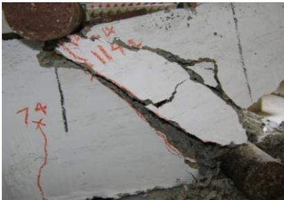
**Fig. 1 Failure mode of shear deficient RC reference beam**
