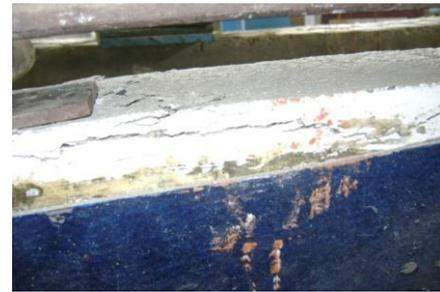
**Fig. 3 Failure mode of U-wrapped beams with symmetric angle-ply laminate**
