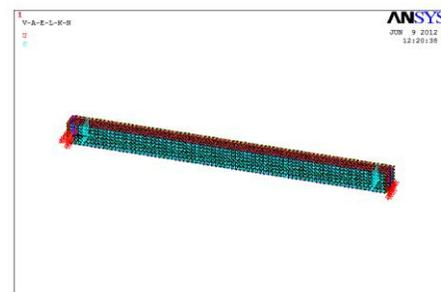
**Fig. 5 Boundary conditions of U-wrapped beam**
